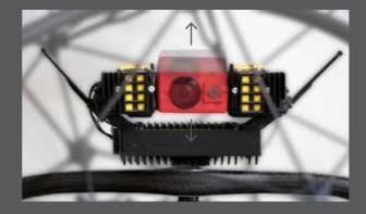
Mounted on a rotatable head the cameras can capture images looking above and below the drone. The full HD camera offers a total field of view of 215° and a horizontal field of view of 130° while the thermal camera offers a total vertical field of view of 182° and a horizontal field of view of 56°.
