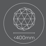
Spherical, the protective frame comes in one size only. With a diameter just below 400 mm, it is slightly smaller than the smallest standard manhole.
