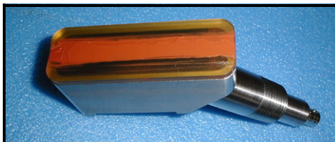
Figure 3-22: Couplant on Transducer Face
