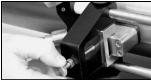
Figure 3-11: Installing the First Transducer
