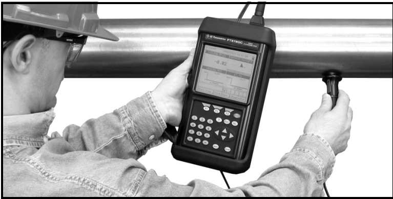
Figure 9-4: PT878GC Thickness Gauge in Operation
