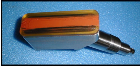
Figure 3-10: Couplant on Transducer Face
