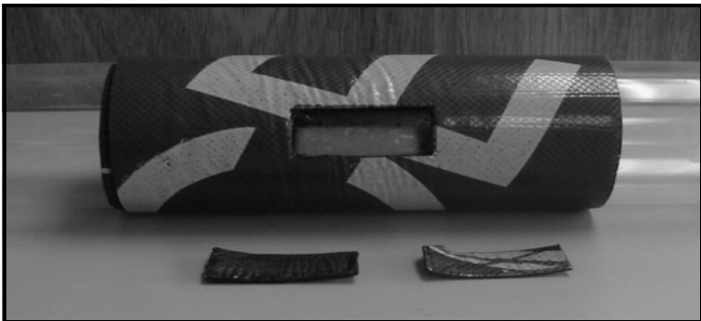
Figure 3-25: DMP-1 Material with Transducer Footprint Cut Out
