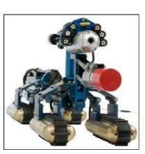
**Sensor Integration**Easy integration such as sonar, NDT sensors, lasers and chemical sensors.
