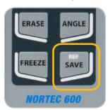
A single press of the new SAVE key instantly stores the current settings (program) and signals (data) in the instrument's memory, together in a single file for maximum convenience and user-friendliness.
