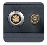
The 16-way LEMO connector also supports the PowerLink NORTEC technology, which features automatic probe recognition and instrument presets for quicker setups.
