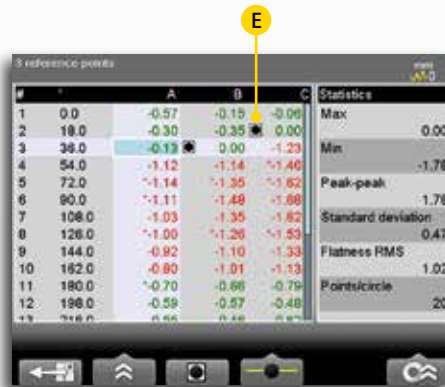
Result table with reference points marked (E). Red values are out of tolerance.
