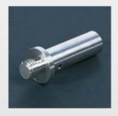
For mounting the D22 transmitter in a spindle (or on a magnet base), for example. Clamping pin diameter 20 mm [0.79"], clamping length 60 mm [2.36"]. Part No. 01-1333
